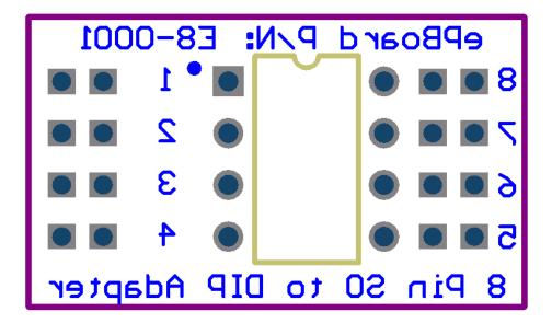
Note: Zero ohm resistor jumpers are mounted on the bottom side to form an eZ-Reconfigurable Adapter. Jumpers can be easily removed and re-wired for different pin connections between top and bottom packages.
